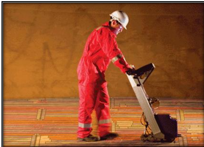
Tank Bottom- Automatic Magnetic Flux Leakage Test
