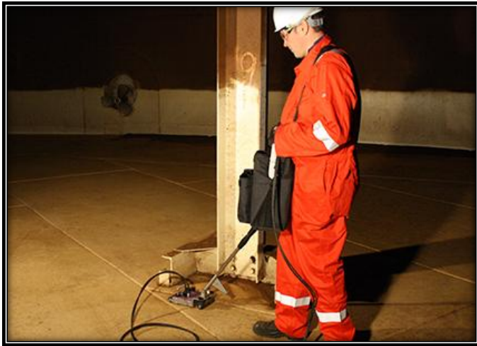
Tank Bottom- Hand Scan Magnetic Flux Leakage Test
